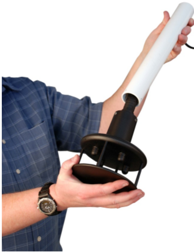
FIGURE 6-17. WindSonic connected to cable
