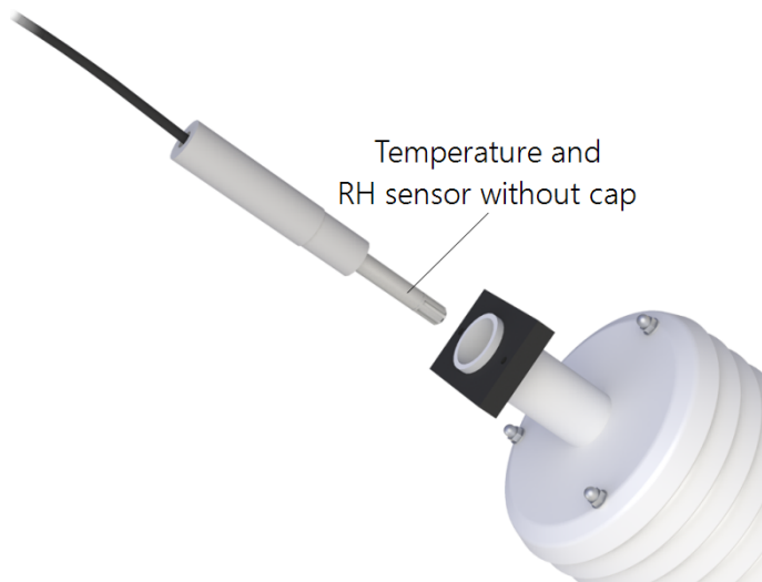
FIGURE 6-10. Temperature/relative humidity sensor without yellow protective cap
