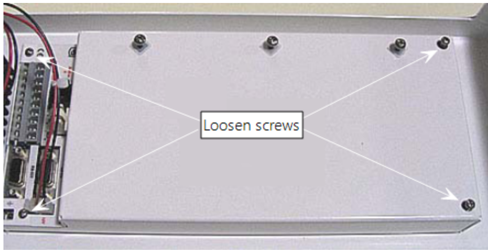
FIGURE 6-13. Screws that secure the electronics cover
