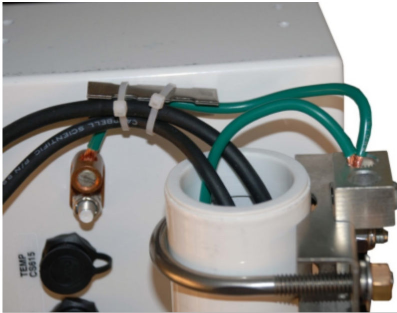
FIGURE 6-41. Grounding to lightning rod clamp
