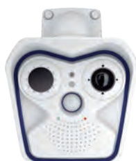
M16-Thermal(-TR) with one add. MX sensor module (Day/Night/LPF, optional)
