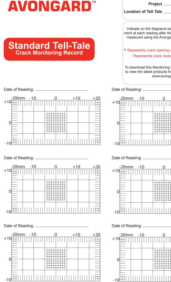
Indicate on the diagrams below the Tell-Tale movement at each reading after the crack widths have been measured using the Avongard Crack Width Gauge. + Represents crack opening and - Represents crack closing on the horizontal scale
