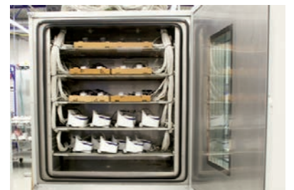
Each camera is tested at extreme temperatures before shipping.
